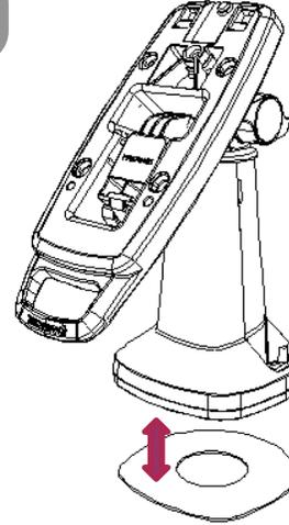
Drill hole to route Cable thru counter 40mm diameter max
